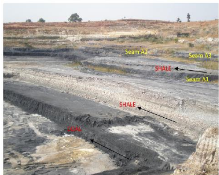
Fig. 7. Maiganga mine in panoramic perspective. A coarsening upward sequence is indicated by the coal seams at the base grade into sandstone, siltstone, and shale (10° 02' 39" N, 11° 12' 17" E)
