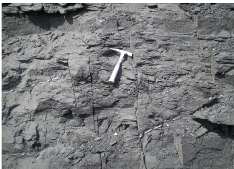
Fig. 9. The dull-lustering, fractured seam B coal at the Maiganga mine is most likely the result of dehydration or stresses in the crust during coalification (10° 02' 39" N, 11° 12' 17" E)
