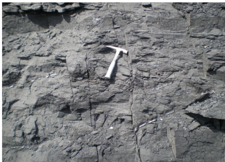
Fig. 9. The dull-lustering, fractured seam B coal at the Maiganga mine is most likely the result of dehydration or stresses in the crust during coalification (10° 02' 39" N, 11° 12' 17" E)
